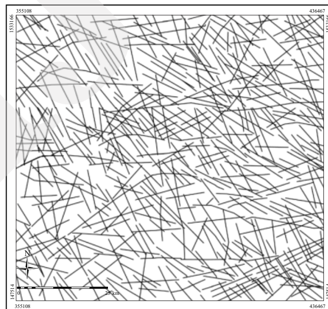
Figure 13. Lineament map extracted from gradient shader image of DEM.
