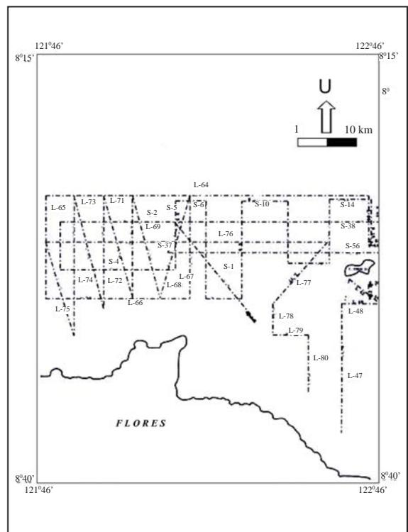
Gambar 3. Peta lintasan seismik pantul.
