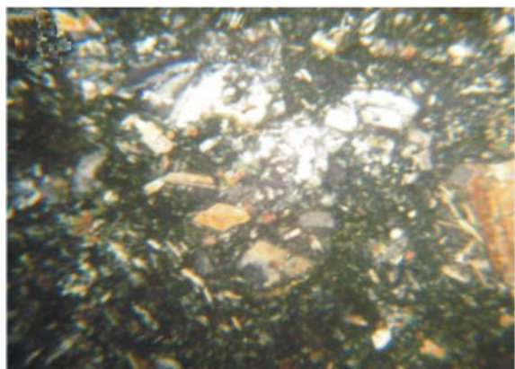
Figure 2. Plagioclase sieve textures in the Cihara Granodiorite.
