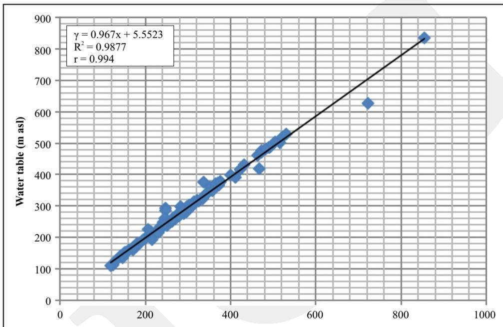
Figure 5. A correlation regression of ground surface elevation vs. water table, indicating an excellent relationship.
