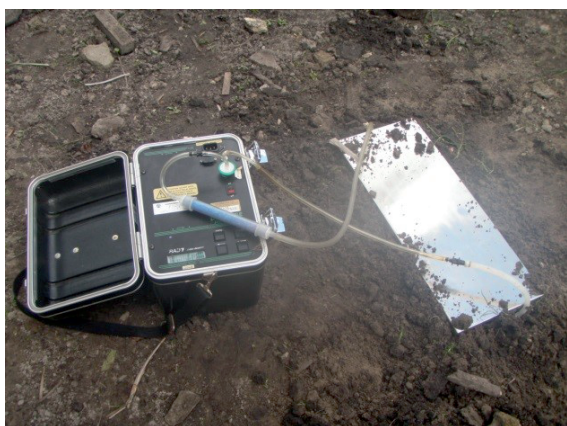
Figure 3. The RAD7 system and accumulation chamber.
