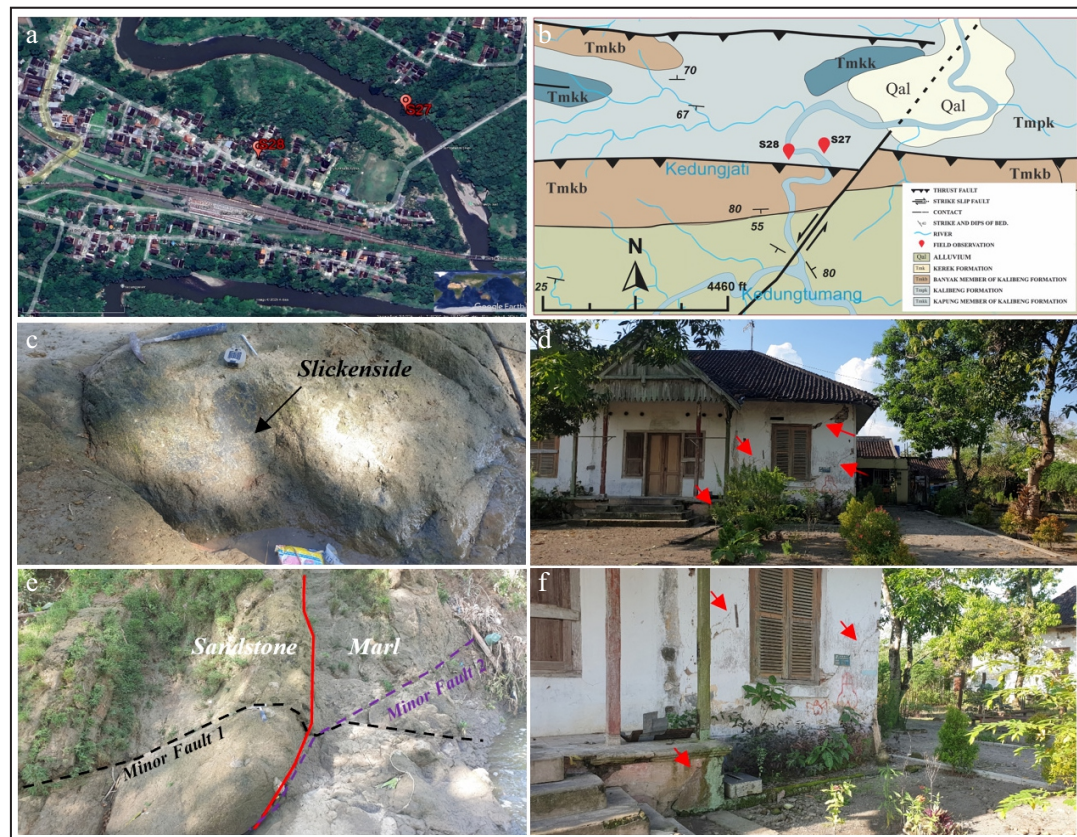
Figure 13. Possible creep manifestation at S27 and S28 stations in Kedungjati Village, image taken from Google Earth on March 3, 2025 (a); S27 and S28 in the Salatiga Geological Map (Sukardi and Budhitisna, 1992), indicating how close these stations are to the major thrust fault (b); fault manifestation at S27 station (c, e), indicating some minor faults; slickenside (c) indicated an E-W direction of N260^{\circ}E with a plane dip of 3^{\circ} . Cracks on old buildings (red arrow) in S28 station (d, f), possibly indicating fault-creep manifestation. These old buildings were built by Dutch officials in 1870.
