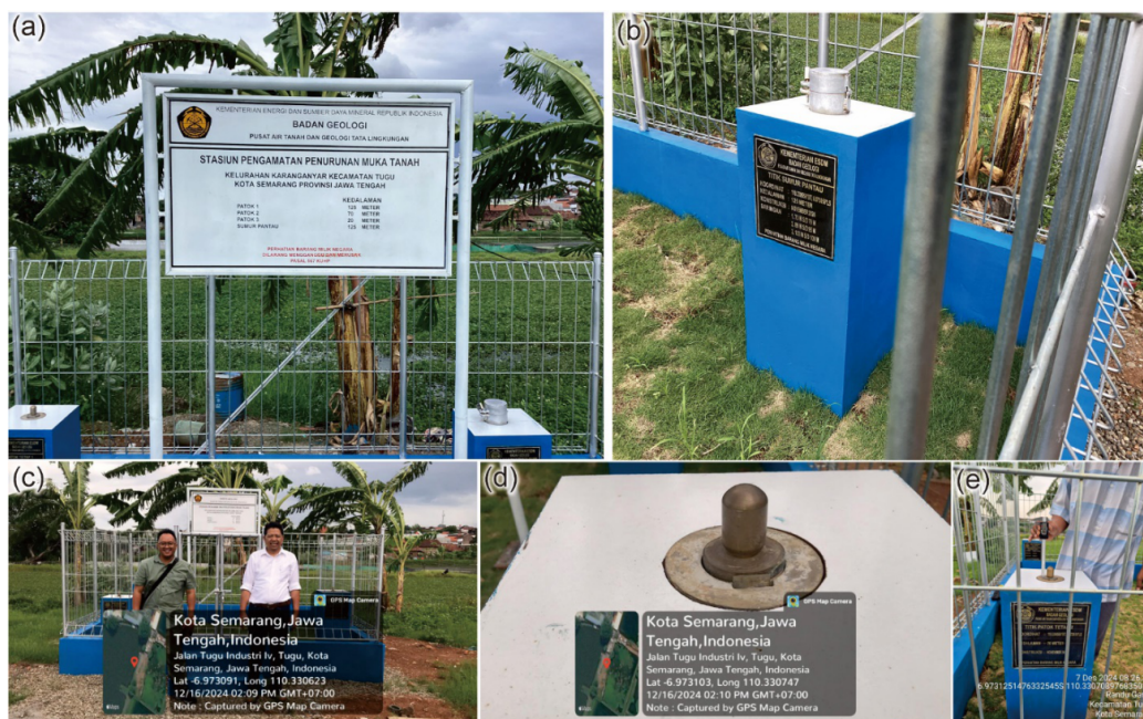
Figure 10. Deep file benchmark monitoring of Tugu Site with different depths, i.e. 125 m, and 20 m. In ten months (November 2024–September 2025), they have shown the value of subsidence until 125 m depth approximately 1.606 cm.
