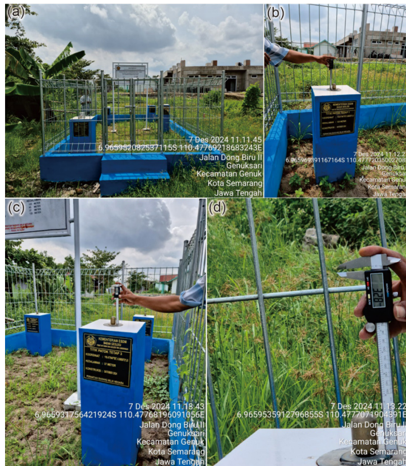
Figure 9. Deep file benchmark monitoring of Genuk Site with different depths, i.e. 85 m and 37 m. In nine months (December 2024 to September 2025), they have shown the value of subsidence until 85 m depth approximately 6.122 cm. (See table 3).
