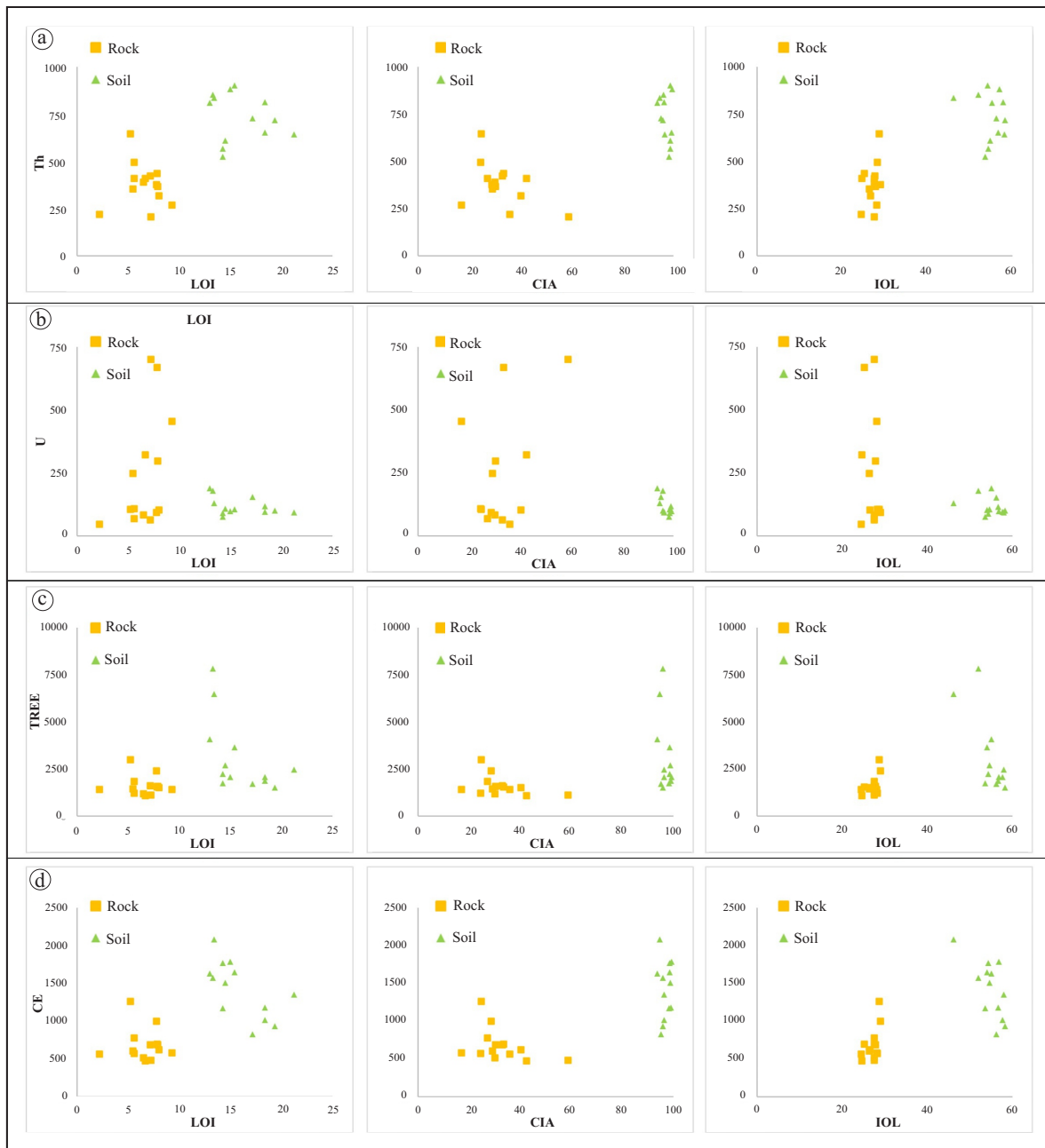
Figure 11. Selected element vs weathering indices: (a) U, (b) Th, (c) Total REE (TREE), and (d) Ce.
