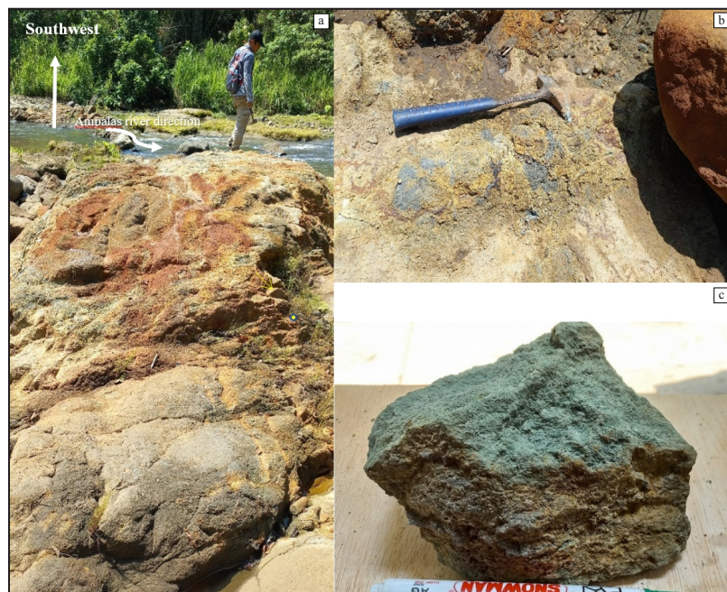
Figure 9. Outcrop of (a) altered foid syenite at the northern part of the studied area for sampling location MMJ603; (b) The presence of secondary minerals in the form of sulfide minerals such as pyrite and chalcopyrite, in dark grey sections; and (c) hand specimen of altered foid syenite in The Ampalas River, Kalukku Subdistrict, West Sulawesi. The sampling locations are depicted in Figure 7a.
