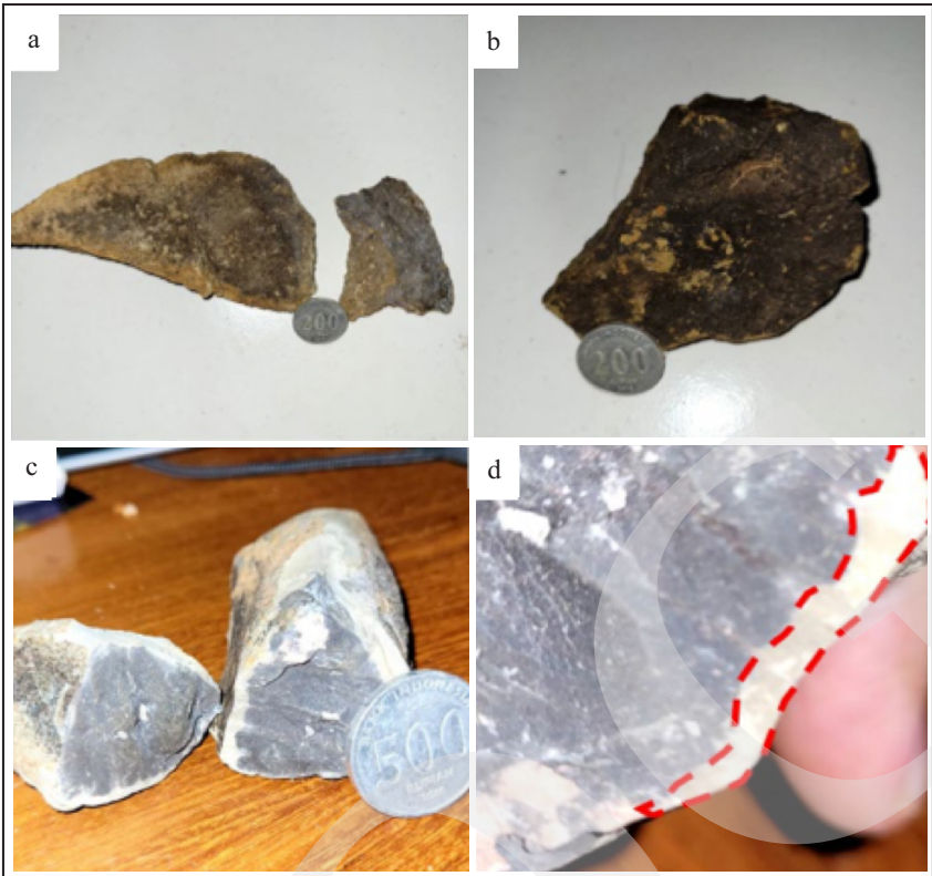
Figure 5. The rock specimens obtained from the outcrops found on SPC-01 comprise (a) Sandstone, (b) Volcanic breccia, (c) Basalt lava, and (d) Volcanic tuff (represented by a red dashed line) that overlays the basalt lava.
