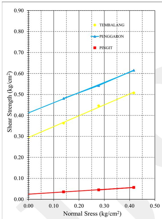
Figure 6. Results of Direct Shear Strength Tests.
