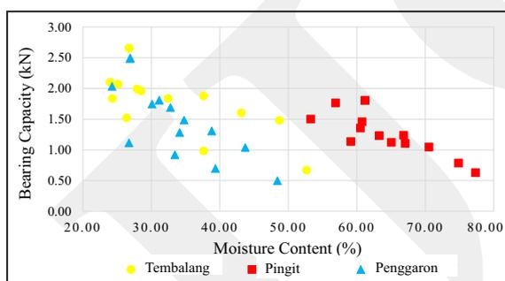
Figure 10. Relationship between Bearing Capacity and Moisture Content
