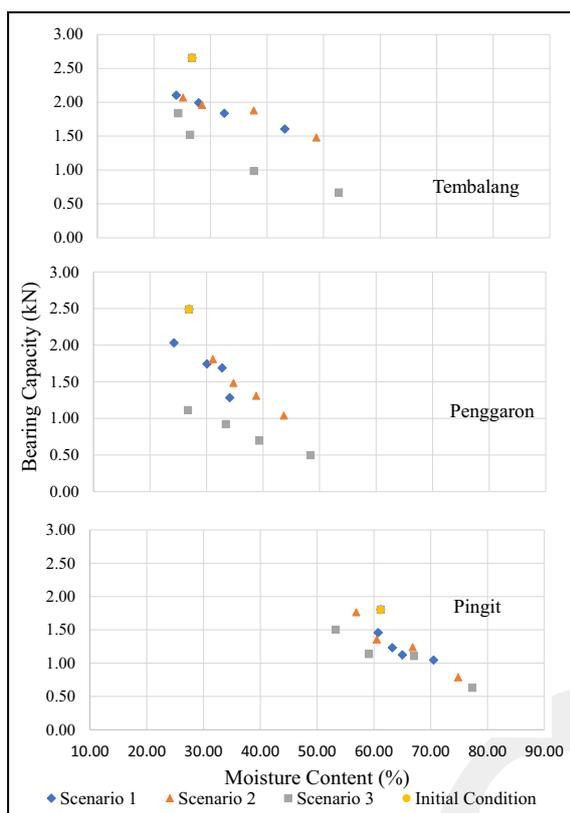
Figure 9. Relationship between Bearing Capacity and Moisture Content. (a) Tembalang (b) Penggaron (c) Pingit.
