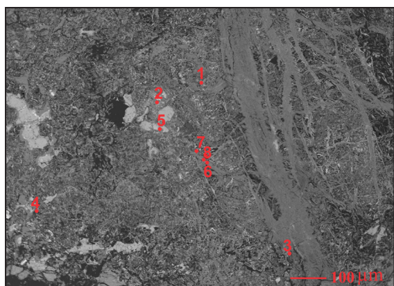
Figure 11. EPMA back-scattered image showing the occurrence of vermiculite (points 1,2,4,5), lizardite (points 3,6), maghemite (point 7), and antigorite (point 8) in the earthy saprolite specimen.
