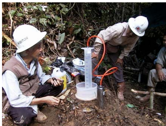
FIGURE 9. PHOTOGRAPH OF IN-SITU GAS IN-PLACE CALCULATION (Q1) OF METHANE GAS, USING A SIMPLE EQUIPMENT IN THE FIELD.
